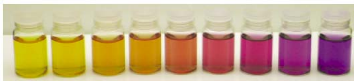
Figure 7 Buffer solutions ranging from pH 7.6 to 9.2 (at intervals of 0.2). 9 cm 3 of each buffer solution was mixed with 1 cm 3 of stock hydrogencarbonate indicator.
