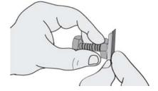
6. Turn the bolt clockwise about 1/12<sup>th</sup> of a turn to make the wax cylinder protrude slightly. Again holding the microtome and blade slice the blade over the nut's surface to make a shaving of the wax surface through the stem. **A smooth quick slicing motion is the best.** Continue the procedure to get several thin sections of the stem.
